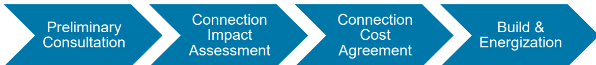
Figure 1: Distributed Energy Resources Connection Process
